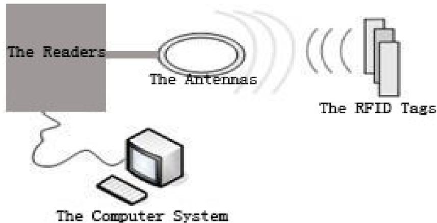
**Figure 4:** RFID system components (adapted from Yan et.al, 2008)
